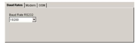
In the register card **baud rates** you may set the transfer rate for the RS232-interface with respect to the chosen transfer route in the communication type.
