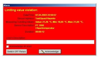
You must enter in the field **user description** a short fault description, to acknowledge an alarm (the entry field is only active with the option PAS-ALARM).
