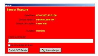
You must enter in the field **user description** short fault description to be able to acknowledge the alarm report (the entry field is only active with the option OP-PANEL/ALARM).
